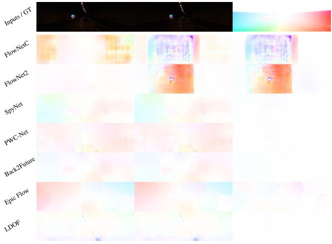
Unattacked FlowAttacked FlowDifferenceFigure 7. Black-box Attacks. Universal patch trained on FlowNet2 and PWC-Net used on all approaches. For this evaluation, we move<br/>the patch according to the static scene.
